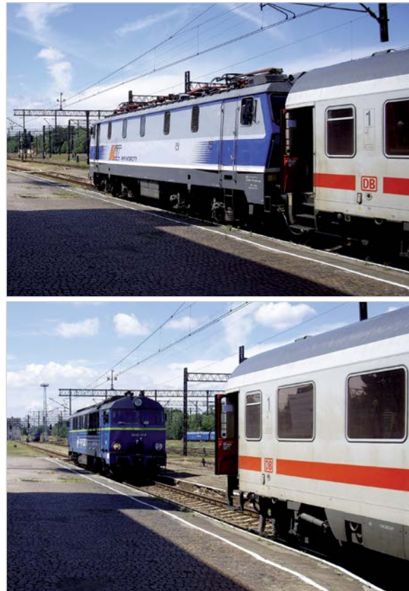
Time-consuming change of locomotives due to lack of electrification – Węglińiec, June 2011 (source: IU / Martin Reents)
